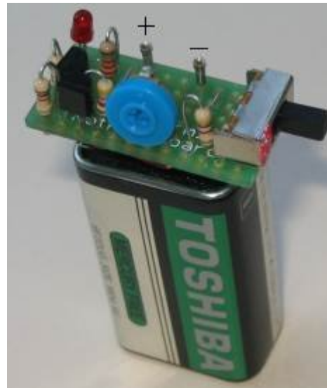
The regulator connected to a 9v battery
